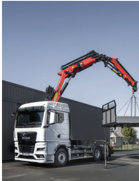
The axle increases the usable capacity and range of cranes.
