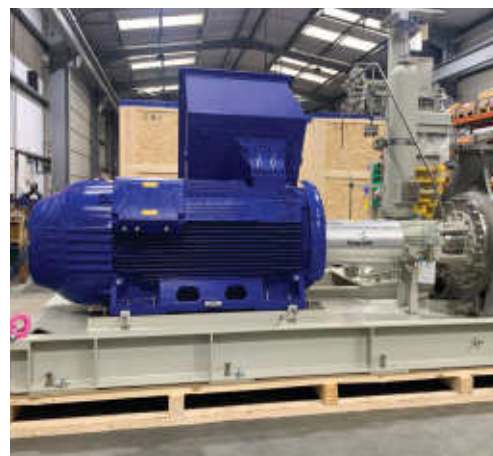
One of the Amarith API 610 OH1 pumps with specialist Plan 53B seal support system.
